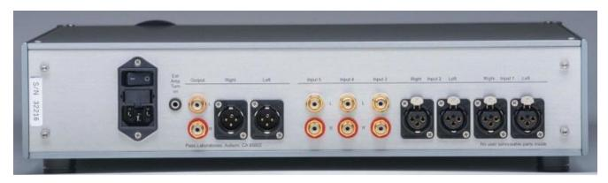
The rear panel has an IEC power cord input with a self-replaceable fuse and the main on/off switch. There are two outputs  $(1 \times RCA)$  and  $(1 \times RCA)$  and five inputs  $(3 \times RCA)$  and  $(2 \times RCA)$ . It also comes with a very nice remote control. As the industry has come to expect from Pass Labs, the build quality is world-class and this preamp looks expensive but not overdone.
